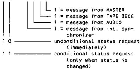
**SBA, SBC** (Status request bytes): SBA contains the basic address, SBC contains the number of bytes of the desired status.
