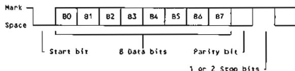
Odd or even parity as well as the number of stop bits (1 or 2) are programmable.
