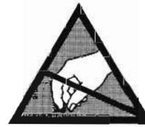
MOS (Metal oxide semiconductor) devices are very sensitive to electrostatic charges. The following precautions should, therefore, be observed:
