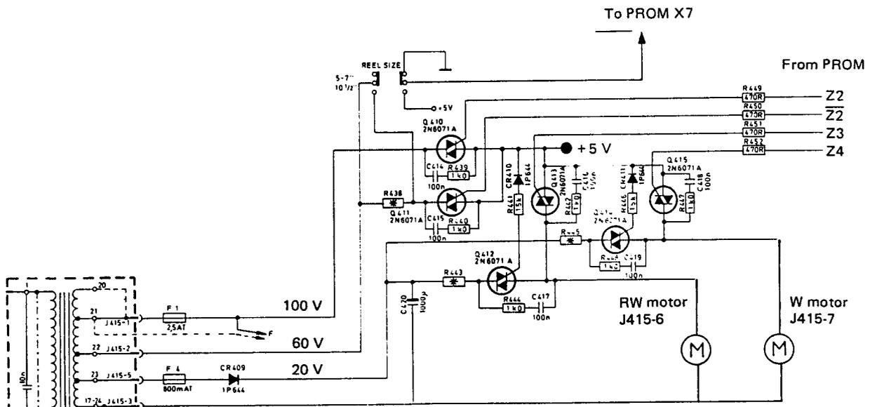
When measuring the voltage in the TRIAC-circuit, the voltmeters — side must be connected to point J415-3.
