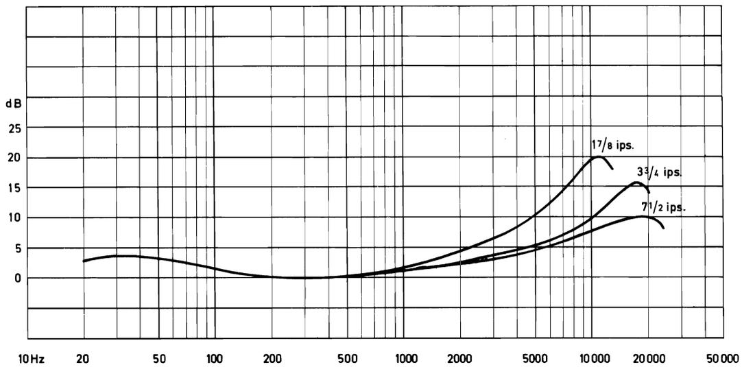
Fig. 4.5 Equalizing curves in record mode
