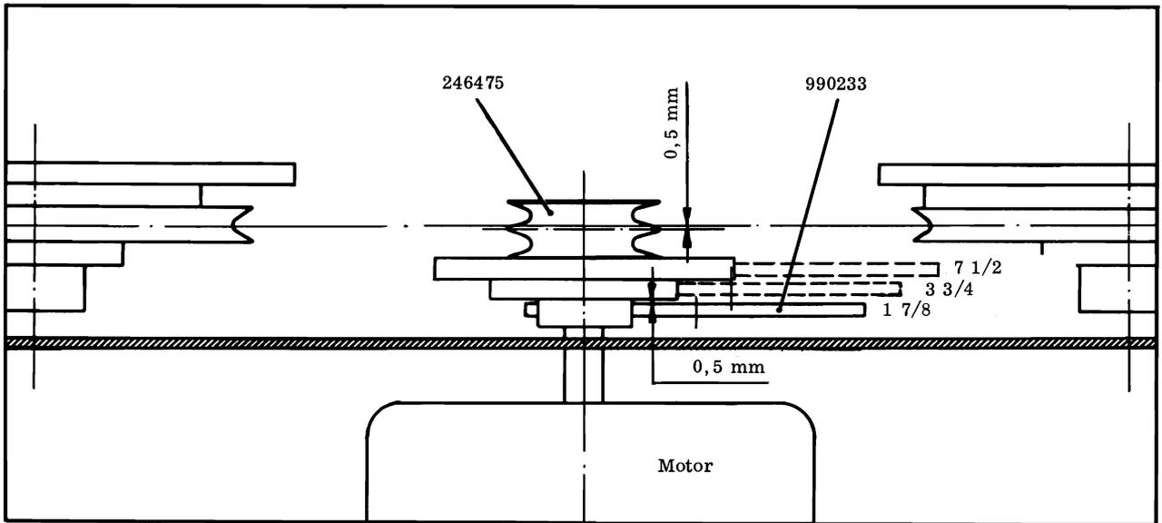
Fig. 3.24 Motor pulley with turntables, rear view
