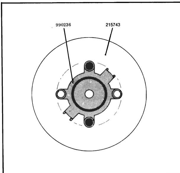
Fig. 3.8 Supply friction disc with mylar sheet
