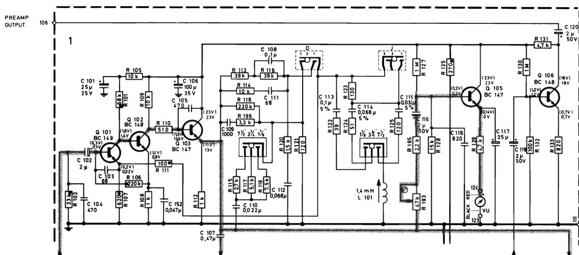
Fig. 4.6 Equalizing amplifier. Signal path in record mode
