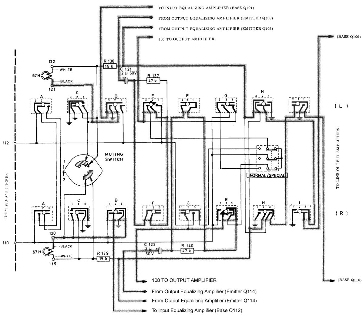
Fig. 4.14 Block diagram and signal path through the switches.
