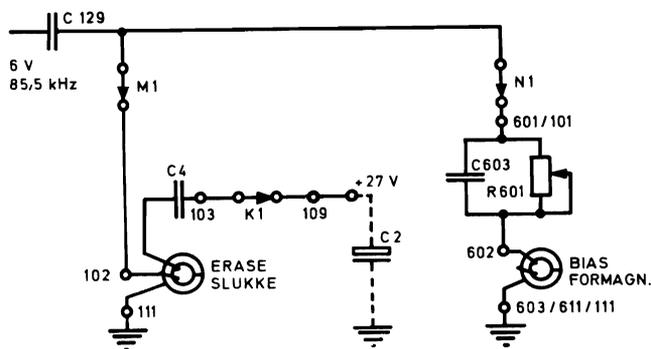
Fig. 4.18 Wiring of erase- and bias heads
