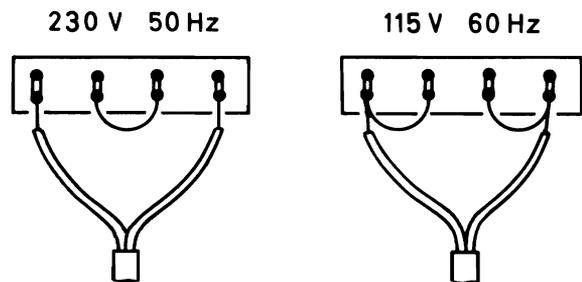
Fig. 6.1 Mains transformer connection.
