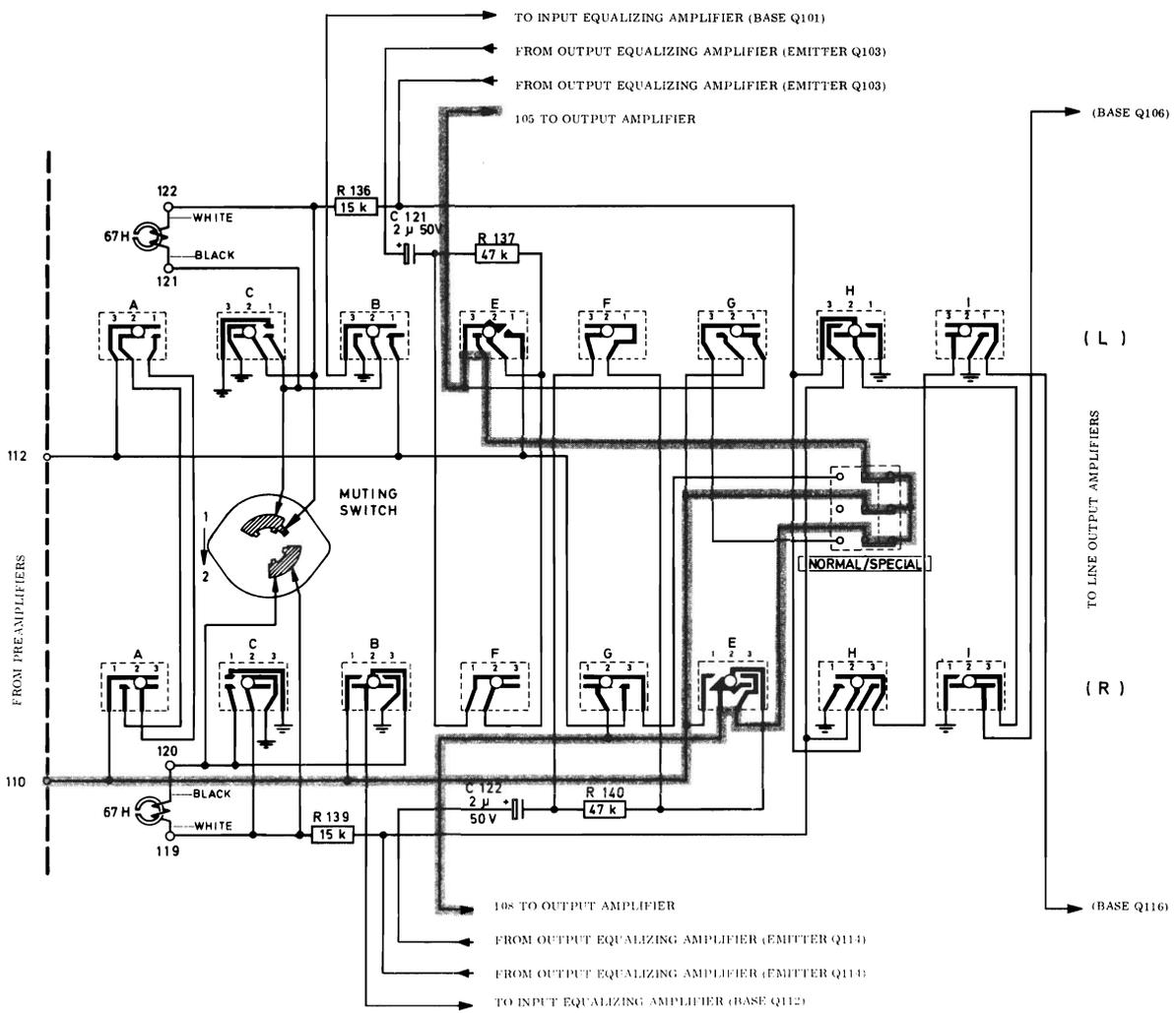
Fig. 4.17 Block diagram and signal path through the switches, L:AMP, R:AMP, SPECIAL
