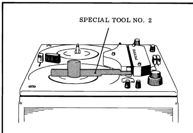
Fig. 3.12 Control of position of turntables
