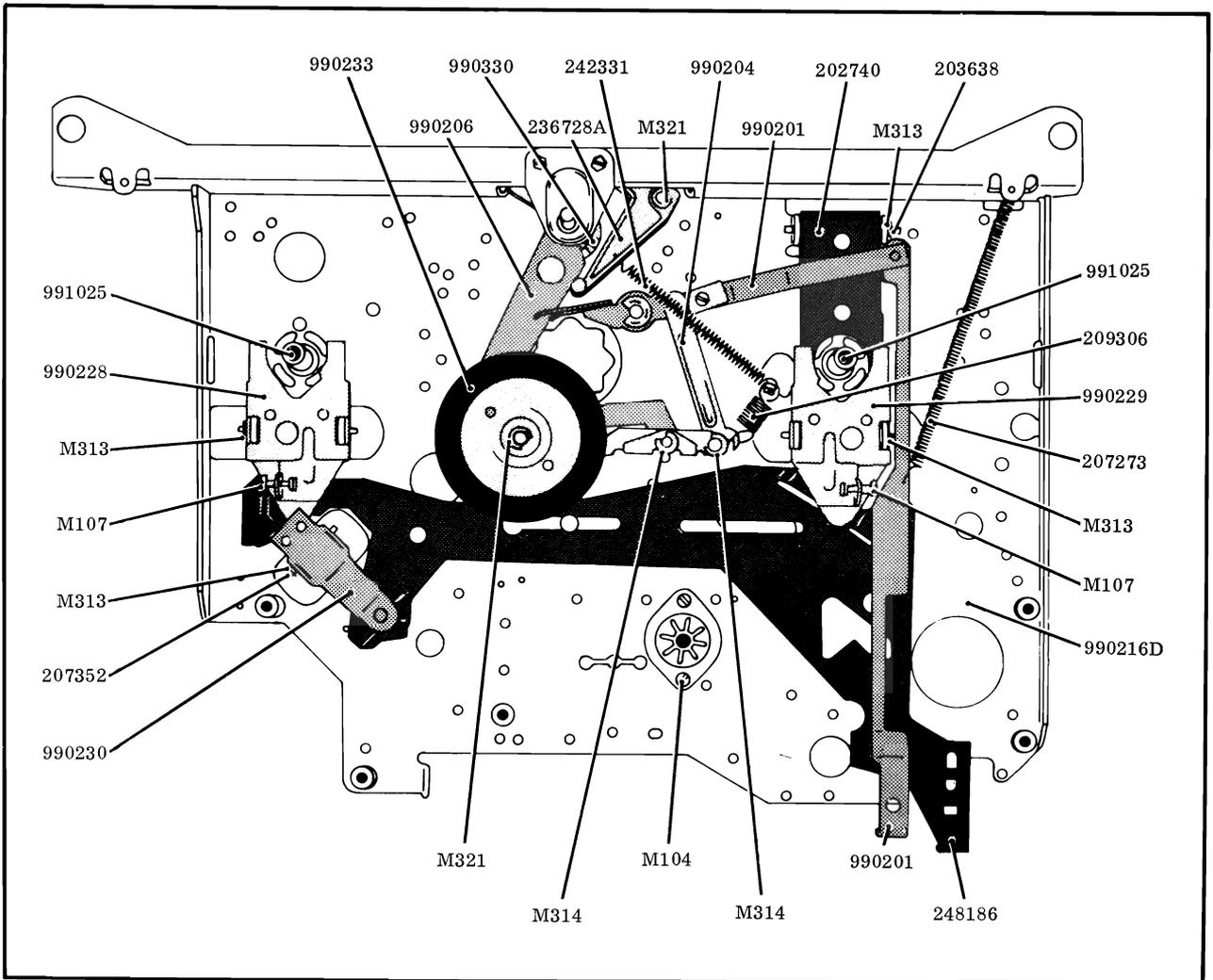
Fig. 3.5 Lower mounting plate
