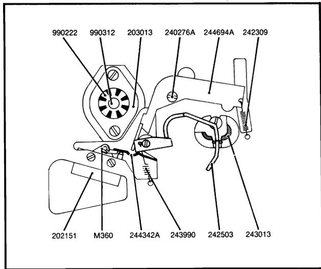
Fig. 3.35 Normal forward drive and fast winding
