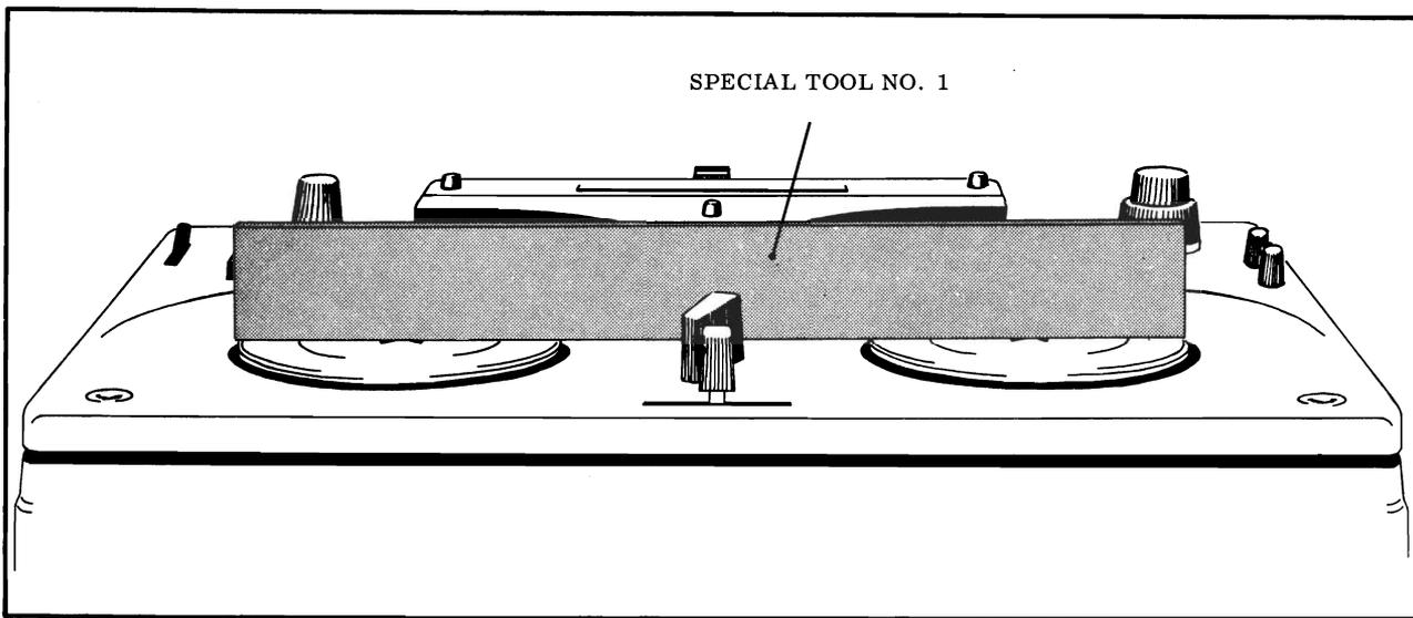
Fig. 3.11 Control of position of turntables
