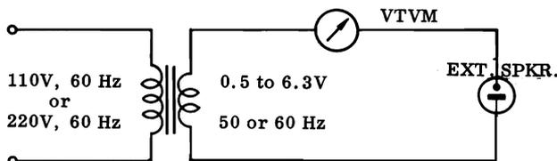
Fig. 5.2 Set-up for tape speed check using VTVM voltmeter.
