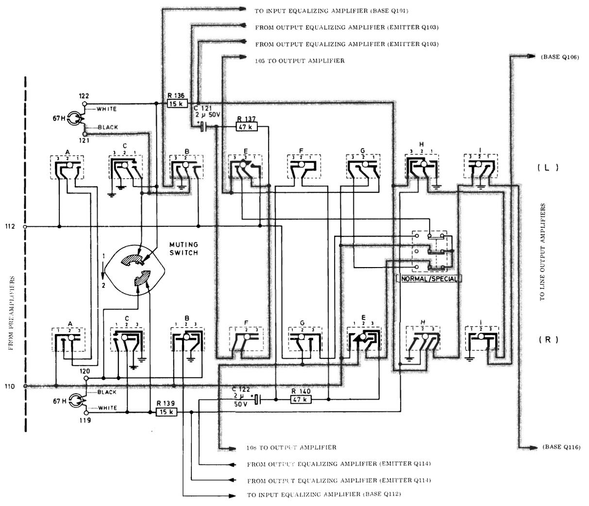
Fig. 4.16 Block diagram and signal path through the switches, L:PLAY, R:AMP, SPECIAL
