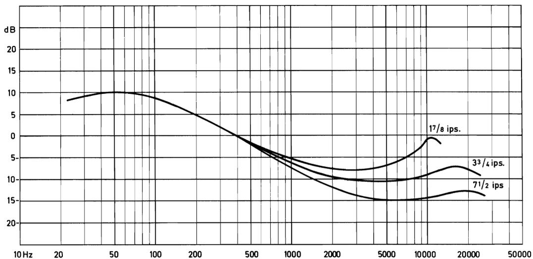
Fig. 4.8 Equalizing curves in playback mode
