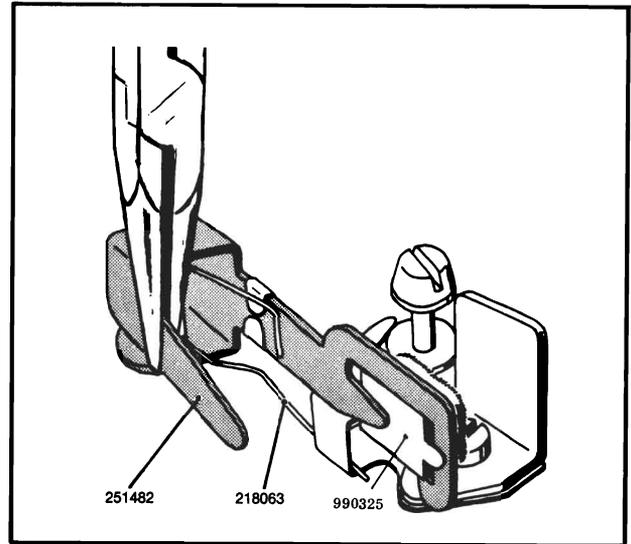
Fig. 3.31 Adjustment of pressure pad
