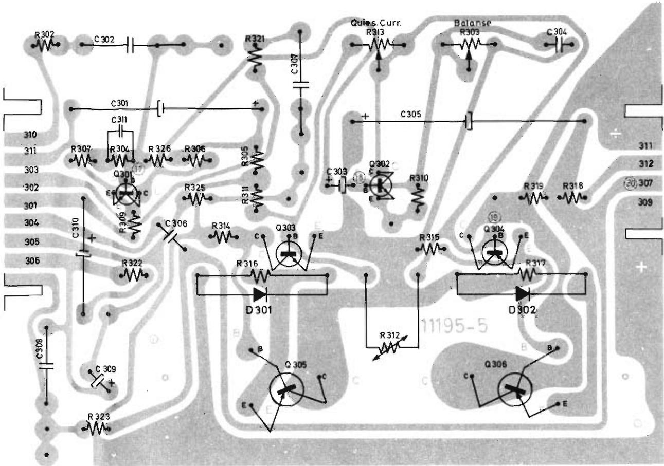
Output amplifier board, seen from printed side
