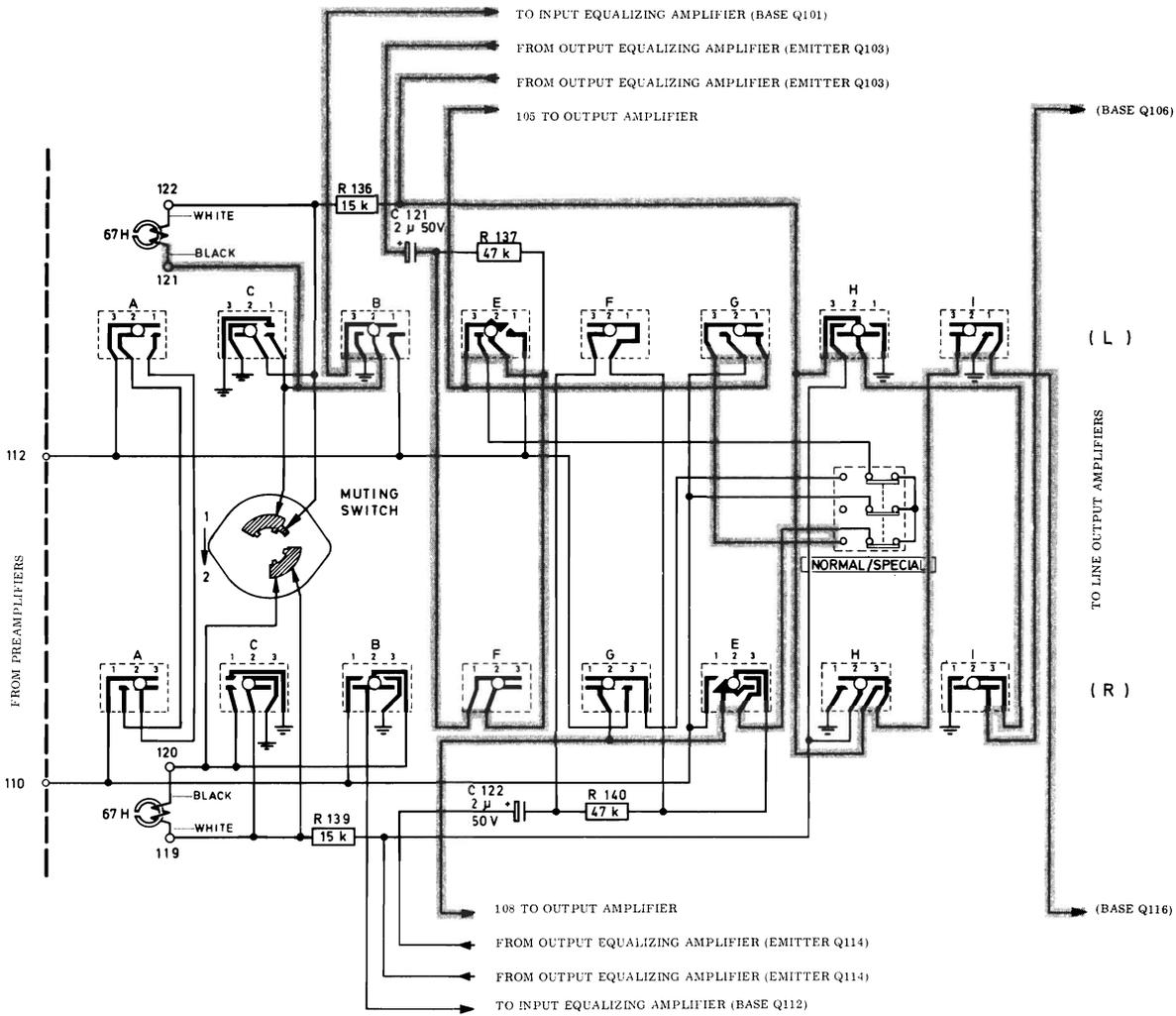
Fig. 4.15 Block diagram and signal path through the switches,
