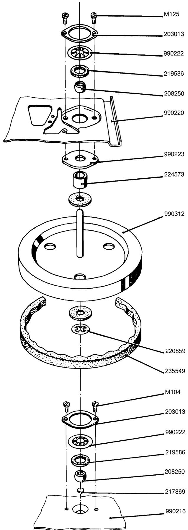
Fig. 4.27 Exploded view of flywheel with bearings.
