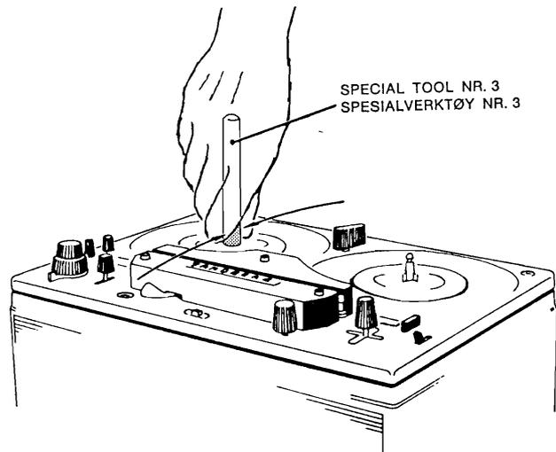
Fig. 4.14 Adjustment of horizontal position.
