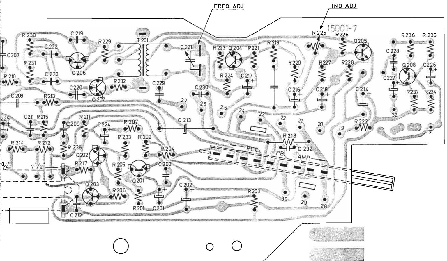
Detector amplifier and oscillator, all models. Seen from print side.
