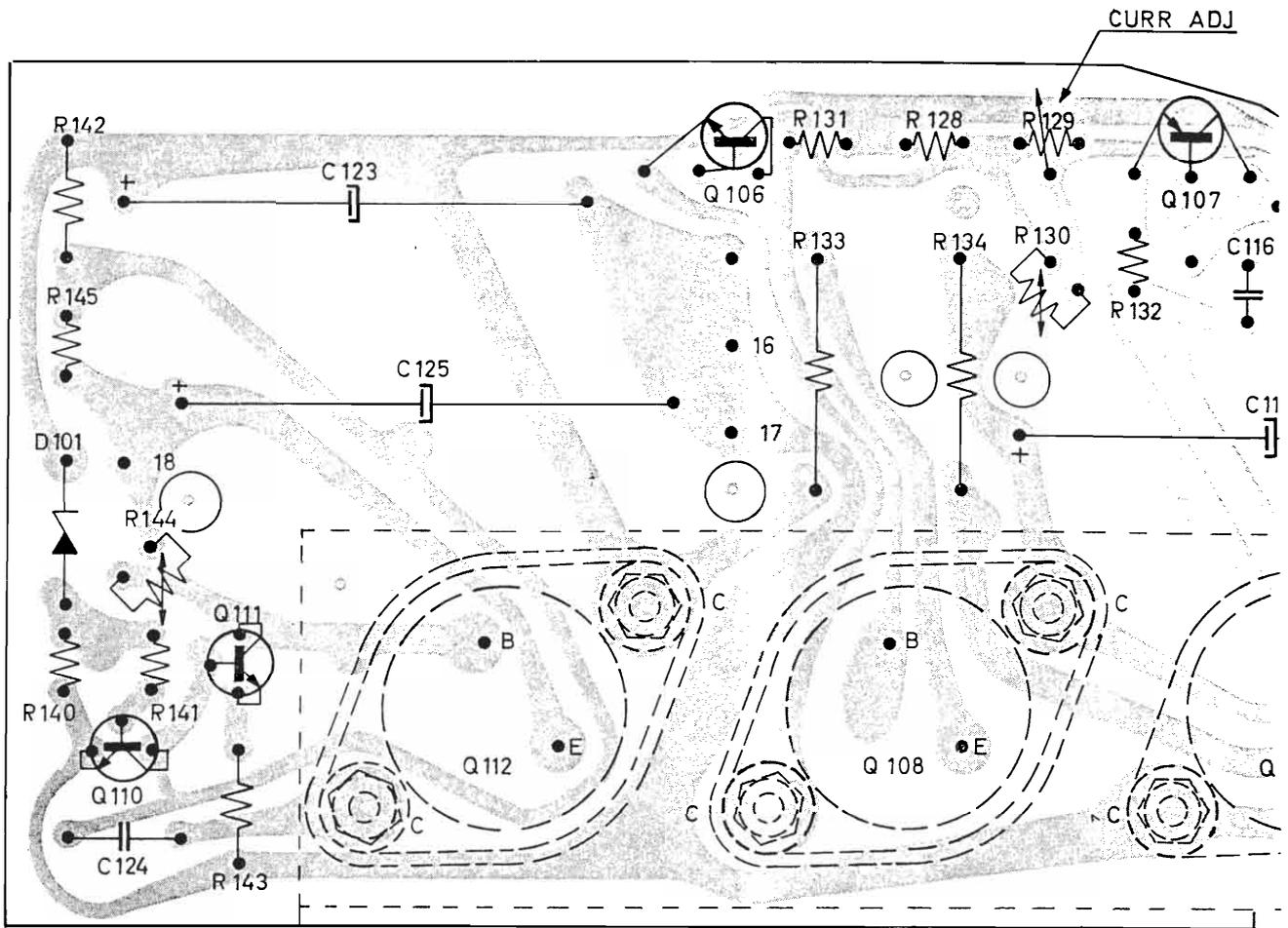
Board for line amplifier, microphone amplifier and voltage regulator, all models. Seen from print side.
