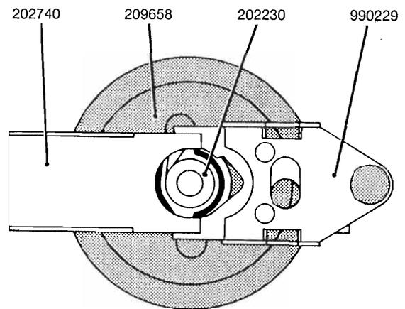
Fig. 4.10 Take-up friction disc with clutch levers.
