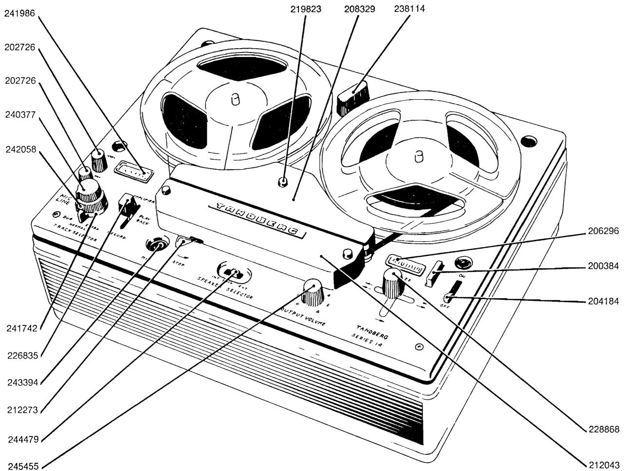
Fig. 4.1 Front top view of the recorder.
