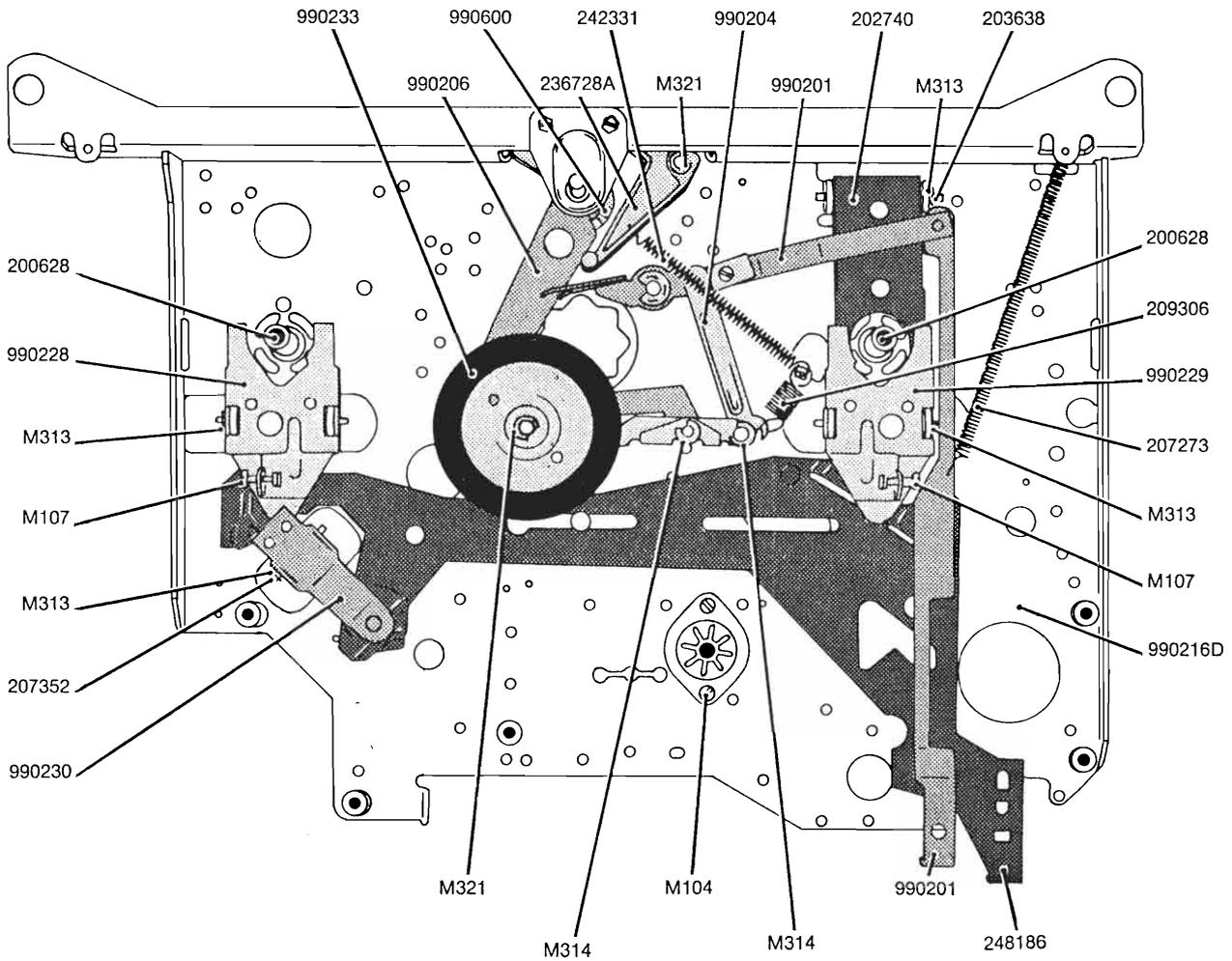
Fig. 4.5 Lower mounting plate with mechanical parts.
