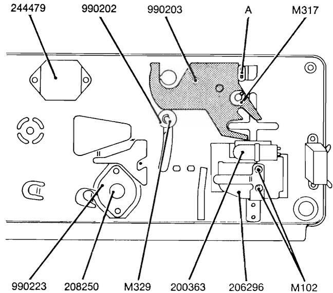
Fig. 4.2 Bottom view of upper mounting plate.
