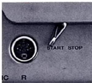
Slide the START/STOP lever to the START position and playback commences. During playback the tape can be instantly stopped and started by using the START/STOP lever.
