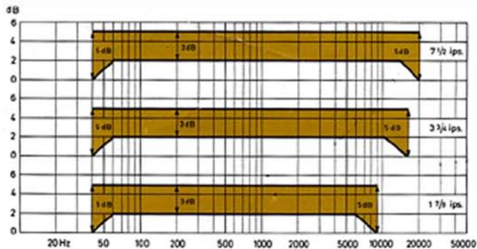
The coloured areas indicate the tolerances for total frequency response according to DIN 45511.
