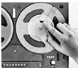
Place the end of the tape in the opening in the empty reel and hold it in place while turning the reel counter-clockwise until the tape is taut.
