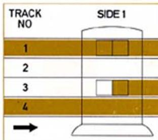
The upper part of the tape head is now disconnected and the lower part is active. The programme is recorded on track 3.
