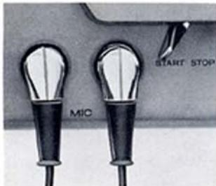
Stereo recording is accomplished in the same manner as described for recording (described on page 7) with the following exceptions should microphones be used: Connect one microphone to the MIC L receptacle and place it to the left of the sound source. Connect the other microphone to the MIC R receptacle and place it to the right of the sound source.
