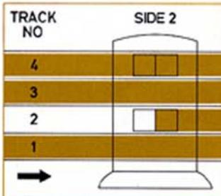
When the complete length of the tape has again been recorded, turn over the tape and continue recording on the right channel. The programme is now recorded on track 2.
