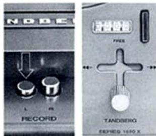
Slide the instantaneous START/STOP lever to the STOP position. Assuming that the recording is to be made on the left channel, depress the RECORD button designated L and hold while setting the tape motion lever in the → position. Should the recording be made on the right channel, depress the RECORD button designated R.
