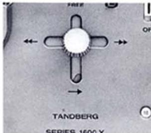
Return the tape motion lever to the center position when the recording is completed. The recording button will then automatically return to the raised position and the machine will be ready for playback.
