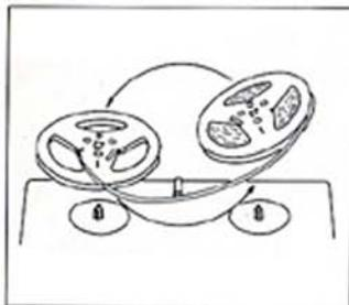
When the complete length of the tape has been recorded and the left reel is empty, turn the tape over, changing turntables. The full reel will now be on the left turntable and side 2 of the tape is ready for recording. For practical purposes the tape is referred to as having a side 1 and a side 2. These are defined as: Side 1: Tracks 1 and 3, side 2: Tracks 4 and 2. In reality only the dull side of the tape is recorded upon.
