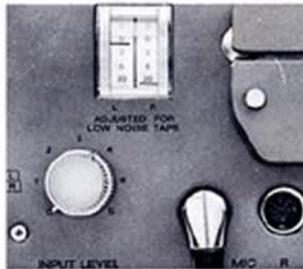
Turn up the INPUT LEVEL knob L until the indicator deflects up to the red field. If the signal is being conveyed through one of the R channel inputs, adjust the recording level with the INPUT LEVEL R knob. It is permissible for the indicator to go into the red field for shorter periods of time but continuous registration in the red field will result in distortion. If the recording level is too low, the result will be an unfavourable signal-to-noise ratio.
