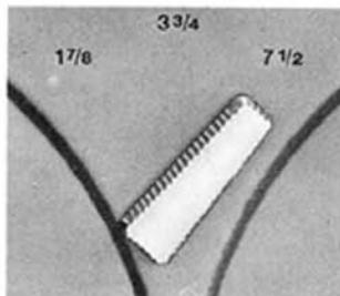
Set the speed selector to the desired speed. The best sound quality is obtained at the highest speed,  $7\frac{1}{2}$  ips. See technical specifications on page 14.
