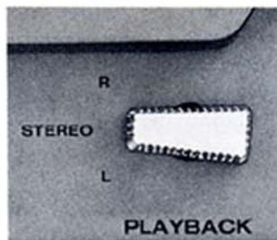
With PLAYBACK selector in the STEREO position two tracks are replayed at the same time. On side 1: Tracks 1 and 3, on side 2: Tracks 4 and 2. The programmes will then be fed separately to their corresponding outputs.
