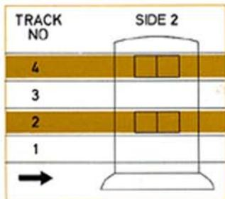
When side 2 is up, track 4 is replayed if the PLAYBACK selector is in the L position, track 2 when the selector is in position R.
