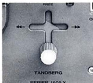
Slide the START/STOP lever to the STOP position and set the tape motion lever in → position.
