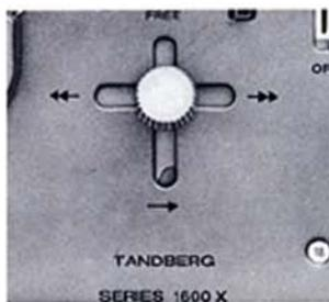
Upon completion of playback return the tape motion lever to the center position. The tape motion lever should be in the center position when the tape recorder is not in use.
