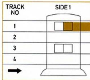
Programmes can be recorded on four separate tracks on 4-track models, with each track covering almost one-fourth of the width of the tape. If a programme is recorded on the left channel, the RECORD L button is depressed and the upper part of the tape head is activated. This programme is recorded on track 1.
