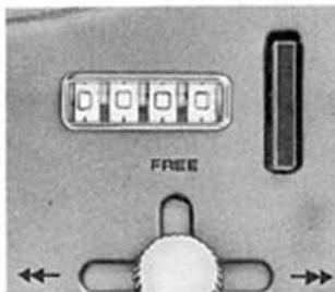
Set the revolution counter to 0 by pressing the reset button. The counter indicates the number of revolutions of the right hand turntable during recording, playback, fast rewind and fast wind, and can be depended upon as long as the inner diameter of the tape reel used on the right turntable is the same.
