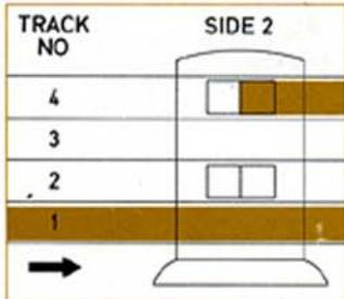
If recording is continued on the left channel, the upper part of the tape head is activated and the programme is recorded on track 4.
