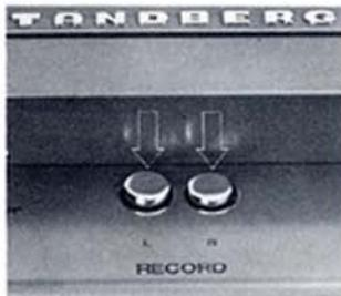
Slide the START/STOP lever to the STOP position. Depress the RECORD L and R buttons and hold while setting the tape motion lever in the → position. Both recording meters will now light up.
