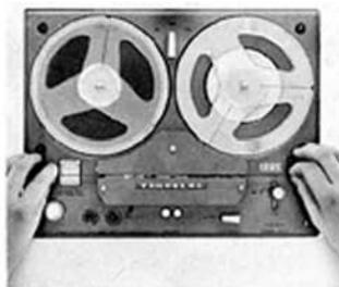
Cut off the adhesive strip at the beginning of new tapes to avoid getting glue on the tape heads. Place a full reel of tape on the left turntable. Hold the tape taut between the left and right hand and lower the tape down into the opening insuring that the shiny side on the tape is towards the front of the machine.
