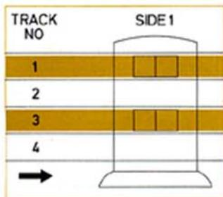
The choice of channel to be replayed is accomplished through the PLAYBACK selector. When side 1 of the tape is up, track 1 is replayed if the PLAYBACK selector is in position L, track 3 when the selector is in the R position.
