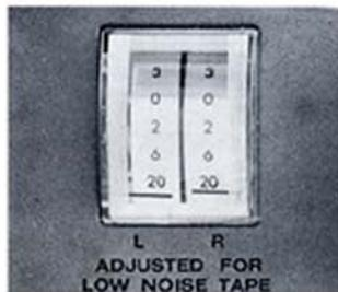
The L recording meter will light up when the left RECORD button is depressed. For recording on the right channel the R recording meter will light up.
