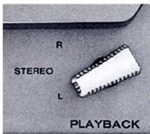
Set the PLAYBACK selector in position L for playback from the left channel. The playback selector has three positions. Position L: left channel connected to both OUTPUT L and R, position R: right channel connected to both OUTPUT L and R, and position STEREO: left and right channels are separated and connected to OUTPUT L and R respectively.
