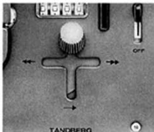
Set the tape motion lever in the FREE position, thereby disengaging both of the turntables from their clutches for easier loading.
