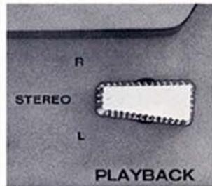
Set the PLAYBACK selector in the STEREO position and slide the START/STOP lever to the START position. The INPUT LEVEL knobs have no influence on the playback signal. Playback level is adjusted by the volume controls on the radio/amplifier.
