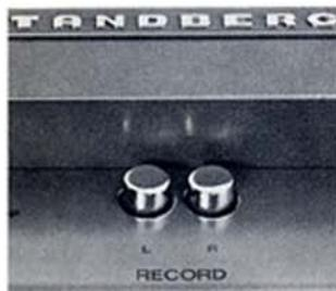
The tape recorder must be connected to a separate radio/amplifier for playback. The RECORD buttons must be in the raised position.
