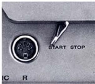
Start the recording by sliding the START/STOP lever to the START position. During recording the tape can be stopped and started instantly by using the START/STOP lever.
