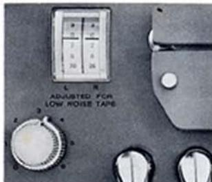
Adjust INPUT LEVEL L and R in the same way as described on page 7. Upper knob: Left meter. Lower knob: Right meter. Slide the START/STOP lever to the start position and commence recording. For recording from another stereo tape recorder or record player the microphones must be disconnected from the machine.
