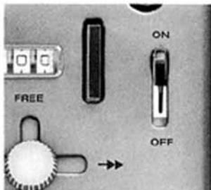
Connect the power cord located in the storage room at the rear of the tape recorder to power outlet. Set the power switch to ON.
