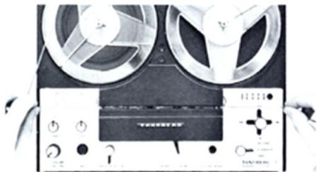
Pull out some tape, hold it tight between the hands and insert it into the slot. Set the operating lever to FREE, to allow the turntables to rotate independently. Insert the tape leader (usually green or red) into the slot of the
