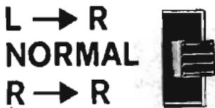
**R → R:** Program from R channel playback amplifier is in sound on sound fed to RADIO input pin 4 by internal connection for recording on L channel. In echo mode, the recording takes place on R channel.
