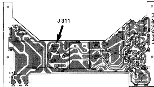
The power supply board seen from the component side.
