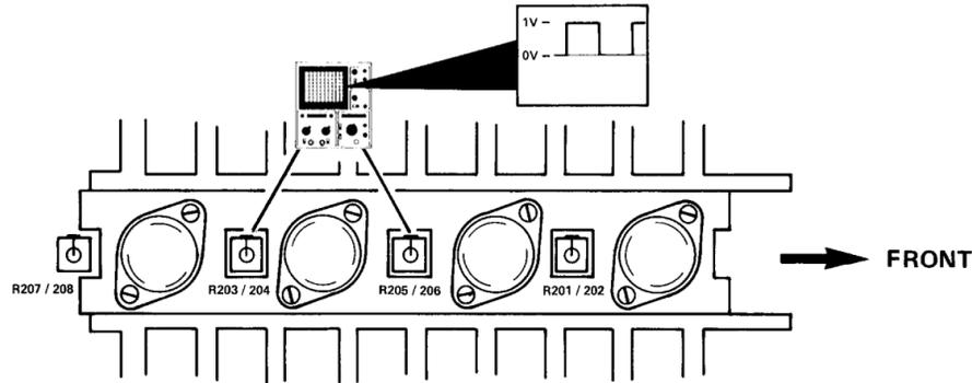
Checking the shortcircuiting protection circuit.
