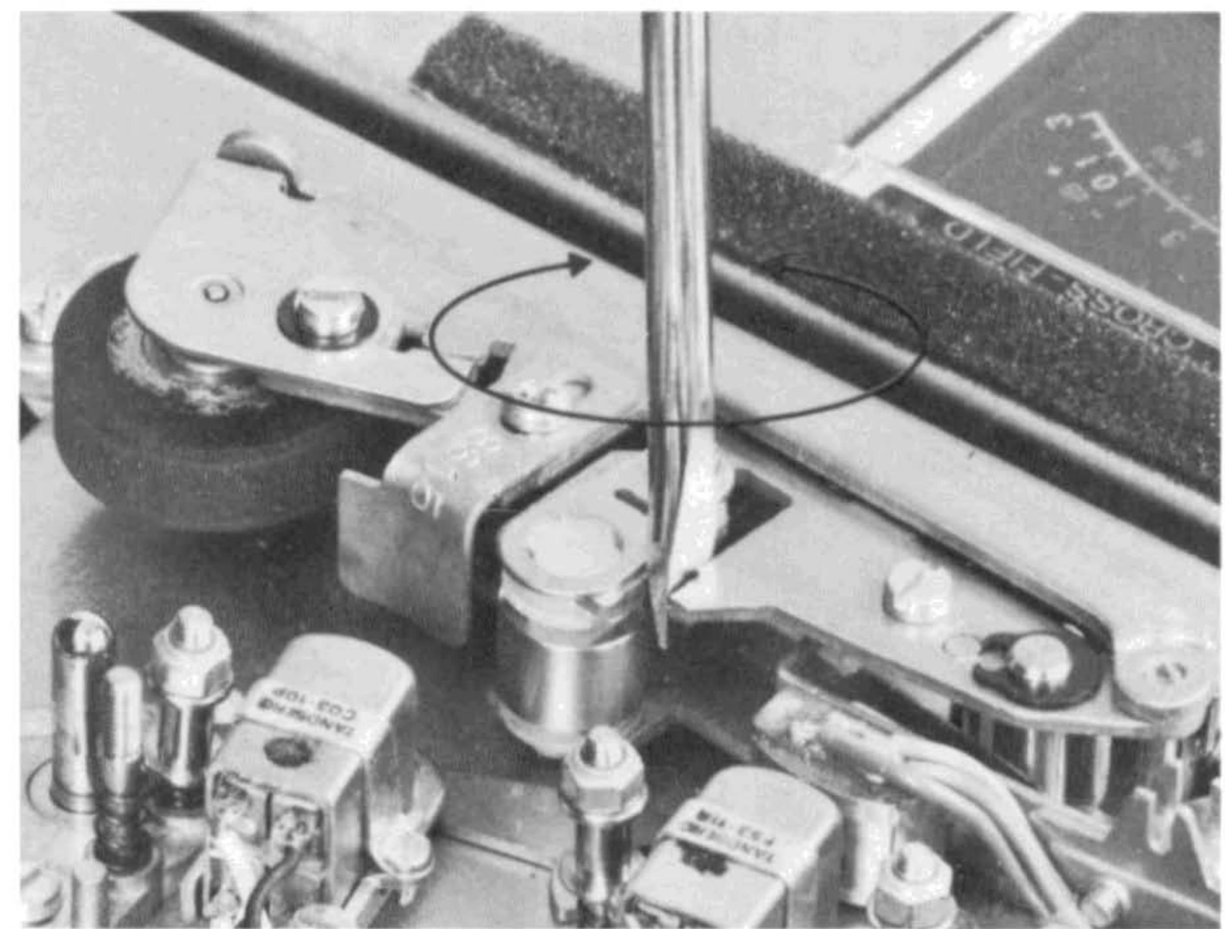
Fig. 2.16. Azimuth adjustment of inertia idling roller.
