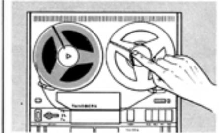
The tape can be threaded with one hand. First, put the tape around the left hand tension arm and position the tape in the slot between the two head covers. Pull the tape around the right tension arm to the take-up turntable. Wrap up a few turns of tape by turning the reel anticlockwise. Select the tape speed. The best sound quality is obtained at 7 1/2 ips, whereas 1 7/8 ips gives the longest playing time.
