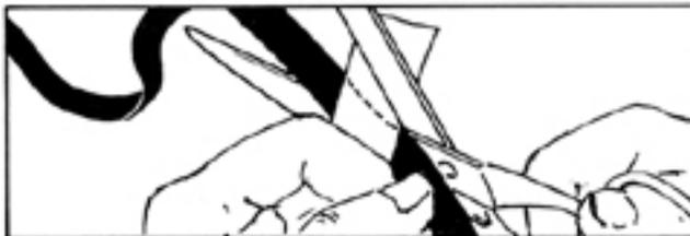
Pull the tape out, and cut it at the mark. Lay the two ends of tape to be spliced over each other with the same side facing up.
