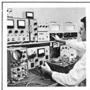
Sample testing. Records taken at random from final production are thoroughly analysed and checked out, with a view to maintaining
