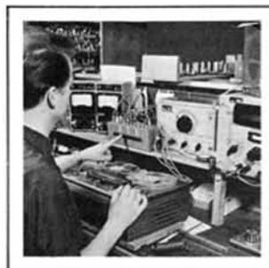
After the final inspection point is passed, every recorder is given a two hour warm up run, and is then given a recheck before pack-
