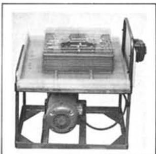
Samples taken from stock are put through some stringent tests. This shows the machine which shakes the recorder very forcibly.
