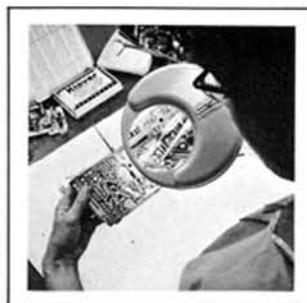
Optical inspection of the printed circuits.
