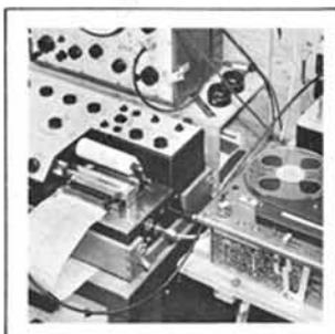
After specially hard handling the recorder is put through a thorough measurement and inspection routine.
