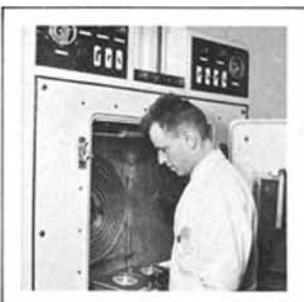
Reliability test in the climate chamber — from arctic cold to tropical humidity.
