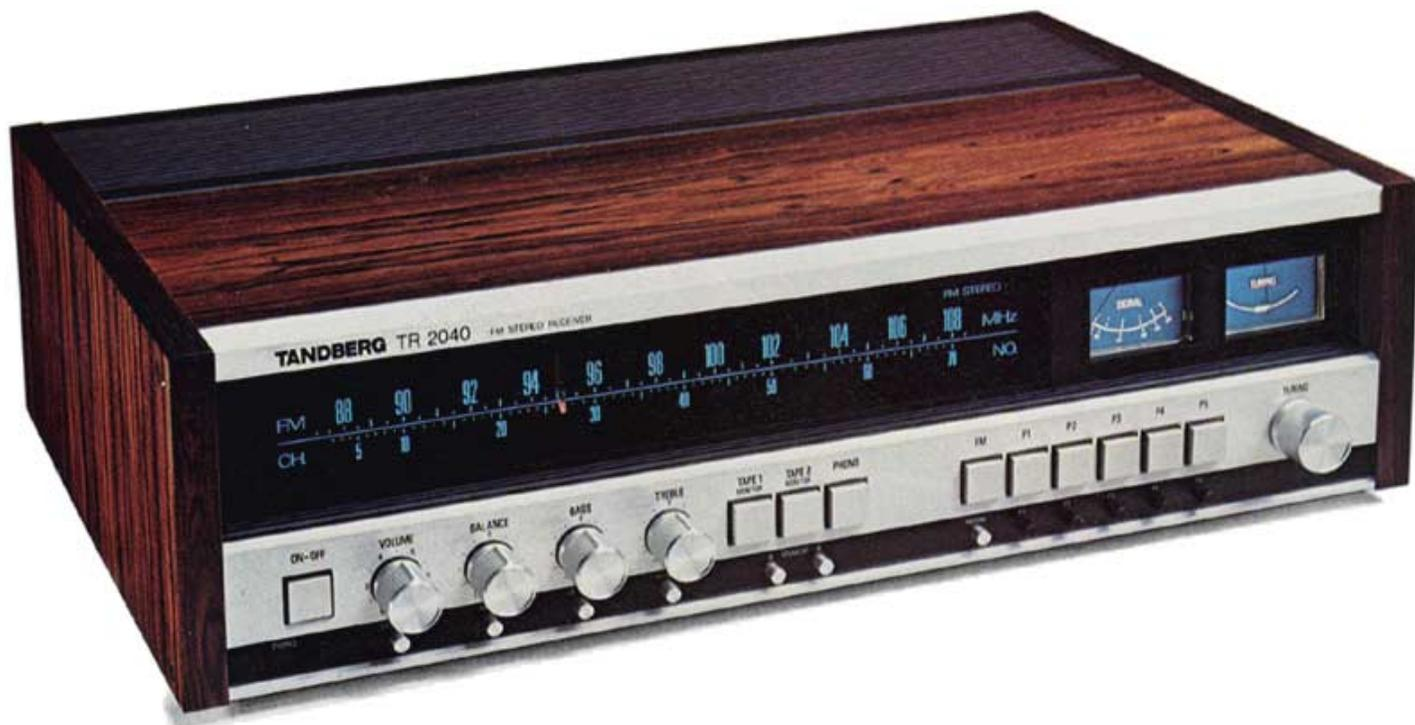
The TR 2040 is also a combined stereo FM receiver and amplifier. The output power exceeds  $2 \times 40$  watts sine wave over the complete frequency range 20 Hz to 20 000 Hz with less than 0.09% total distortion. The output power into 4 ohms is more than  $2 \times 70$  watts sine wave, measured according to DIN! The FM receiver has 5 pre-tune station buttons.
