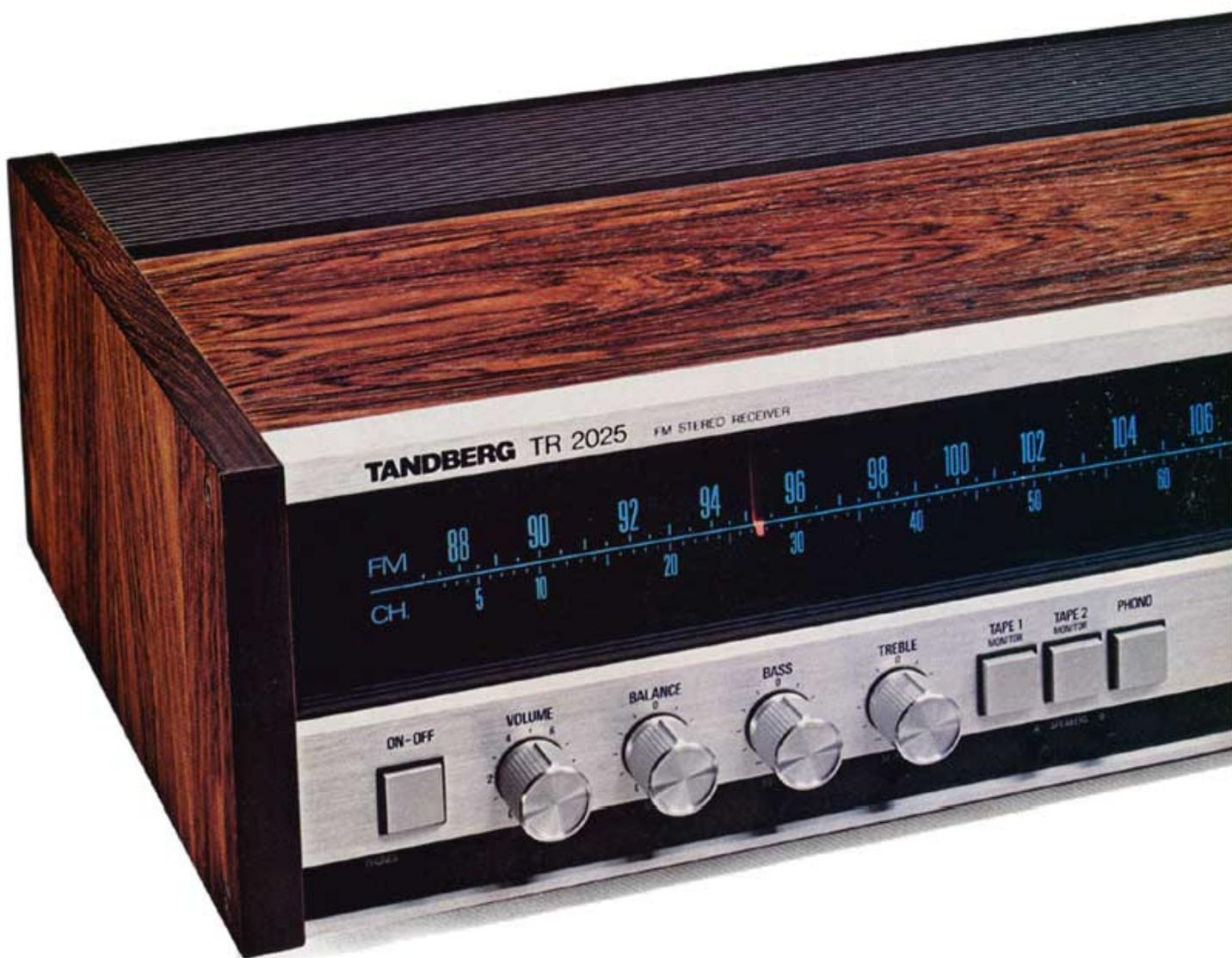
The TR 2025 completes the TR 2000 series — 3 top models to meet a variety of needs and pockets. The stereo FM section has pre-tuning for 5 stations. The power amplifiers deliver more than  $2 \times 25$  watts sine wave in 8 ohms over the complete frequency range from 20 to 20 000 Hz with less than 0.09% total distortion. The output power exceeds  $2 \times 40$  watts in 4 ohms, measured according to DIN!
