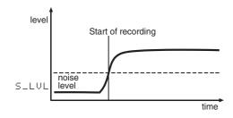
To start synchronized recording when the source is stopped or in pause mode:
