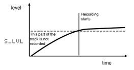
Also remember that when recording from an analog source, the threshold should be set so that it is higher than the "noise floor" (the base level of hiss, pops and crackles which may come from an older vinyl recording, for example). If the "noise floor" is higher than the threshold, synchronized recording will not take place.
