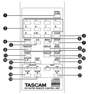
**OPEN/CLOSE key** Opens and closes the disc tray (equivalent to (3)).
