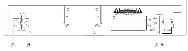
ANALOG IN (L, R) These RCA jacks accept analog audio signals from suitably-equipped units (-10dBV, unbalanced).
