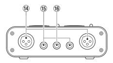
(14) MIC IN (L, R) jacks (XLR balanced) These are analog mic input jacks. The wiring is as follows: pin 1 = ground, pin 2 =hot, pin 3 = cold.
