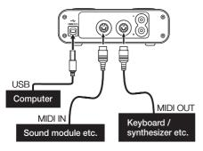
You can use the **MIDI IN/MIDI OUT** connectors to transmit and receive MTC (MIDI Time Code). This allows the MTCcompatible DAW (Digital Audio Workstation) computer application to synchronize with your MIDI equipment.
