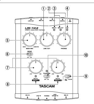
(1) **LINE OUT level knob** Controls the output level of the **LINE OUT** jacks.
