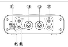
(1) **USB connector** Use a USB cable to connect this to the host computer's USB 2.0 port.
