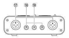
**MIC IN (L, R) jacks** (XLR balanced) These are analog mic input jacks. The wiring is as follows: pin 1 = ground, pin 2 =hot, pin 3 = cold.
