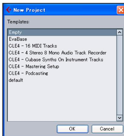
The system displays a window that enables you to select a template for your new project. Select the desired template and press the *OK* button. The system displays the Select directly window. Specify the directory in which you wish to save the project, then click the *OK* button. The new project will be created.
