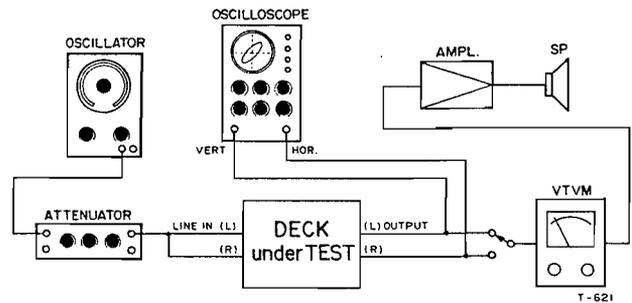
Fig. 8-9 Test Connection for Recording Check
