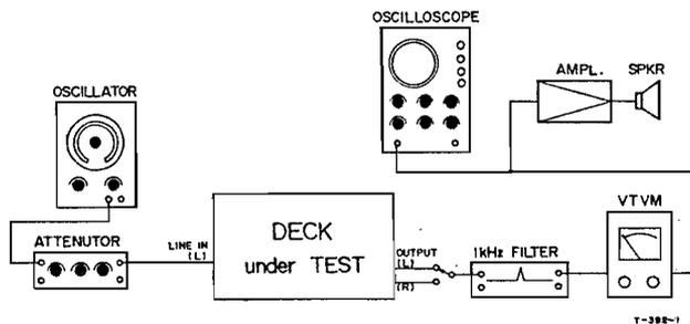
Fig. 8-13 Test Connections for Channel separation check
