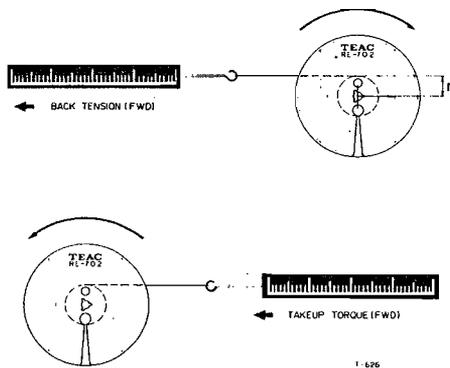
Fig. 7-3 Torque Measurement
