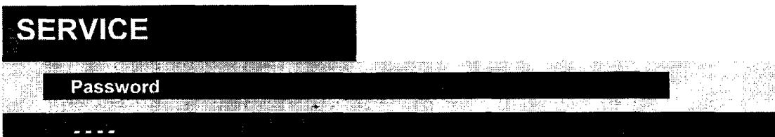
If the password is okay then extra *three* lines will appear as "new password", "hotel mode" and "store." The user will be able to change the password via the first new line, and can store it by accessing the "store" line, as the confirmation of the new password. To change the hotel mode, the user do not have to store it ,i.e, as soon as s/he close the menu, the mode will be the same as s/he did.
