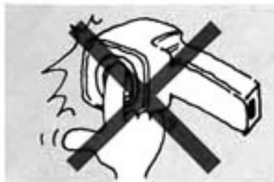
Never touch the discharge terminal and current collector. This may cause performance deterioration.
