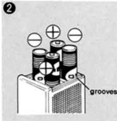
Place dry batteries as illustrated in the diagram. To close battery lid, fit it into the grooves of the body and slide it shut.
