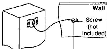
**Screw the wood screw into a thick and hard part of the wall**
