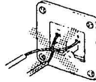
1. Twist the core of the connection cables.
