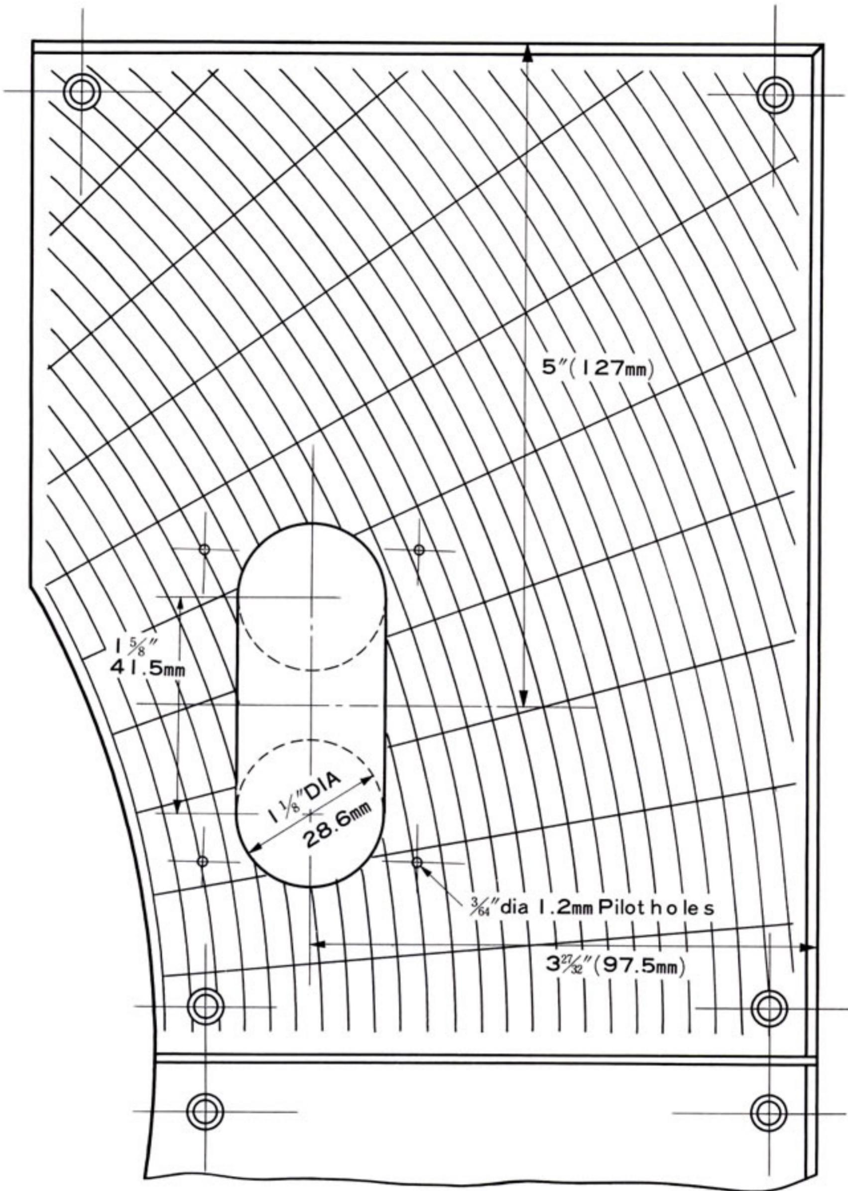
TEMPLATE FOR THE ASSEMBLY OF SME 3009-II IMPROVED PRECISION TONEARM WITH THE SL-110 / DIRECT DRIVE PLAYER SYSTEM.
