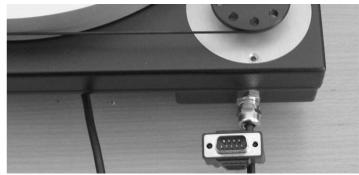
position and the speed selector is on 33 rpm. Then plug in the 3-pin connector from the external AC/AC adaptor to the plug on the back of the PS800. Then connect the main
