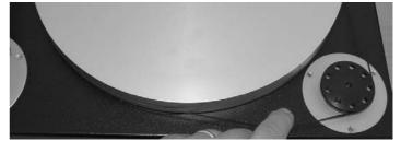
Now place the turntable platter with his axle over the bearing and let it slide into it. Take care that the front end of the axle is not crashing onto the bearing bottom. Then place the rubber belt around the platter and the motor. Now put the feltmat on the platter
