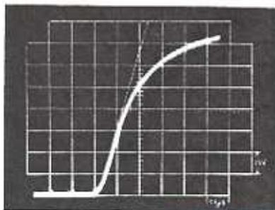
Figure 10 shows the phase deviation with frequency. The direct-coupled amplifier in the DC position gives negligible deviation down to DC. In the NORMAL position, the absence of a sub-sonic filter in this amplifier means that there is only a slight low frequency 'droop' and only +40° phase deviation at 10Hz. At high frequencies, the fact that a two-stage structure is used gives an outstandingly low phase deviation of only -30° at 100kHz.
