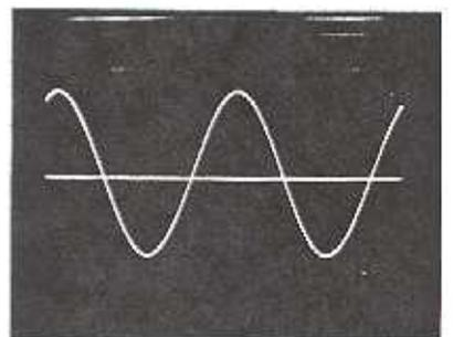
This is clearly attributable to the use of FETs with highly linear characteristics, a sophisticated method for matching pairs, and the symmetrical push-pull drive, etc. The 20Hz waveform, in particular, reveals no ripple content, showing the inherent quality of this DC amplifier.
