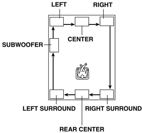
The test tone is heard from the left main speaker, center speaker, right main speaker, right rear speaker, rear center speaker, left rear speaker and subwoofer in order. The tone is produced for 2.5 seconds each time.
