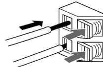
**3** Release the tab to fix the lead wires.
