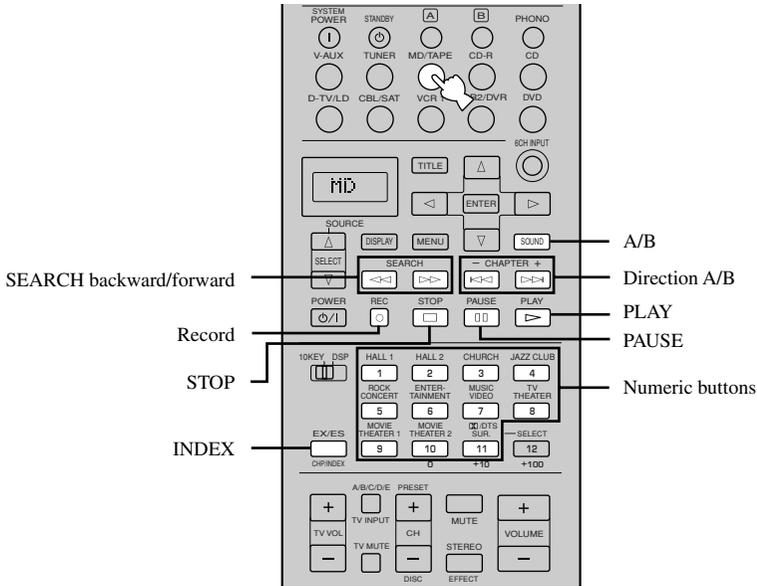
\* TV VOL +/-, TV INPUT, and TV MUTE function to operate your TV without switching the input if the manufacturer code is set in D-TV/LD or PHONO. When the manufacturer code for your TV is set up in the both D-TV/LD and PHONO areas, priority is given to the signal in the D-TV/LD area.
