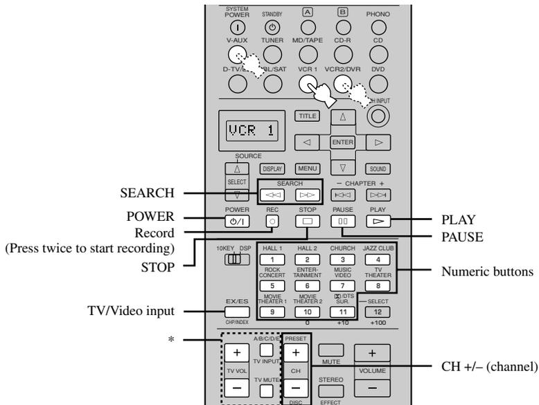
\* TV VOL +/-, TV INPUT, and TV MUTE function to operate your TV without switching the input if the manufacturer code is set in D-TV/LD or PHONO. When the manufacturer code for your TV is set up in the both D-TV/LD and PHONO areas, priority is given to the signal in the D-TV/LD area.
