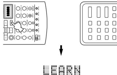
**6** Press and hold the button on the other remote control that has the function you want to program into this remote control until “OK” appears in the display window.
