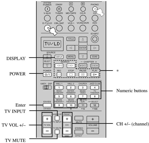
\* SEARCH, REC, STOP, PAUSE and PLAY function to operate your VCR without switching the input to VCR 1 if the manufacturer code is set in VCR 1.
