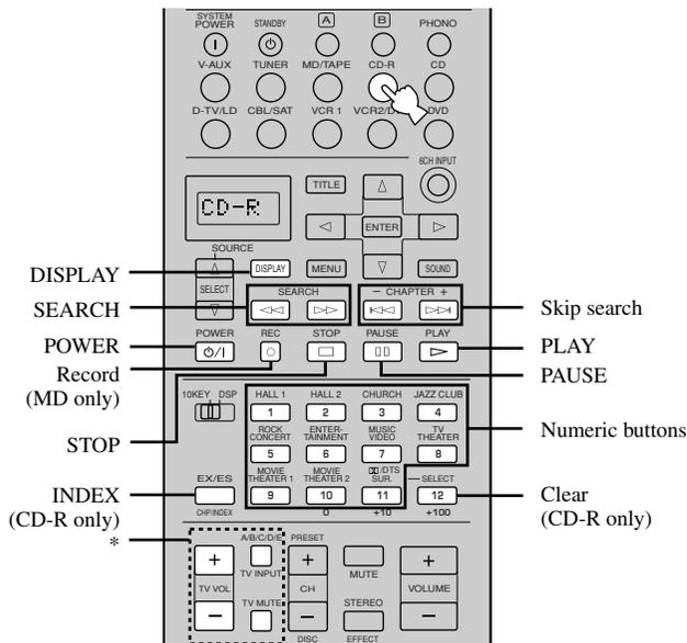
\* TV VOL +/-, TV INPUT, and TV MUTE function to operate your TV without switching the input if the manufacturer code is set in D-TV/LD or PHONO. When the manufacturer code for your TV is set up in the both D-TV/LD and PHONO areas, priority is given to the signal in the D-TV/LD area.
