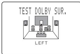
Front panel display also indicates from which speaker the test tone is output in the order of TEST LEFT→TEST CENTER→TEST RIGHT→TEST R SUR.→TEST REAR CNTR→TEST L SUR.→TEST SUBWOOFER
