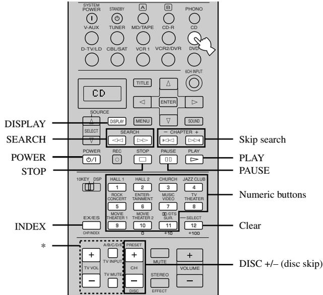
\* TV VOL +/-, TV INPUT, and TV MUTE function to operate your TV without switching the input if the manufacturer code is set in D-TV/LD or PHONO. When the manufacturer code for your TV is set up in the both D-TV/LD and PHONO areas, priority is given to the signal in the D-TV/LD area.
