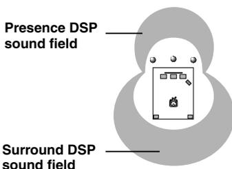
Most movie software has 4-channel (left, center, right and surround) sound information encoded by Dolby Surround matrix processing and stored on the left and right tracks. These signals are processed by the Dolby Pro Logic decoder. The MOVIE THEATER programs for 2-channel sources are designed to recreate the spaciousness and delicate nuances of sound that tend to be lost in the encoding and decoding processes.
