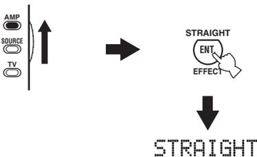
**2** To deactivate the “STRAIGHT” mode, press STRAIGHT on the remote control again so that “STRAIGHT” disappears from the front panel display.
