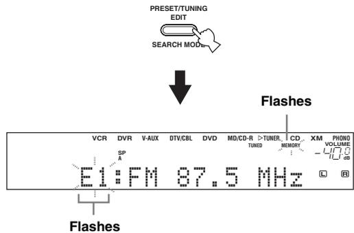
**3 Select preset station “A5” using A/B/C/D/E and PRESET/TUNING/CH </>.**
