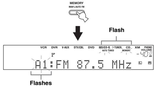
When automatic preset tuning is completed, the front panel display shows the frequency of the last preset station.
