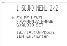
**5 Press ^/∨ repeatedly and then press ENTER to select and enter the desired submenu.**
