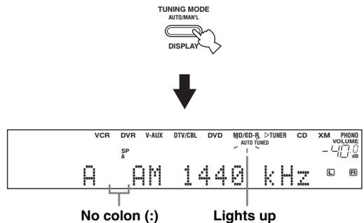
If a colon (:) appears in the front panel display, tuning is not possible. Press PRESET/TUNING (EDIT) to turn the colon (:) off.
