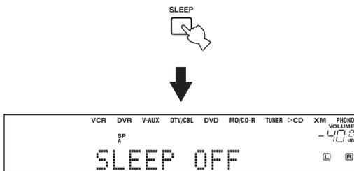
The SLEEP indicator turns off, and "SLEEP OFF" disappears from the front panel display after a few seconds.
