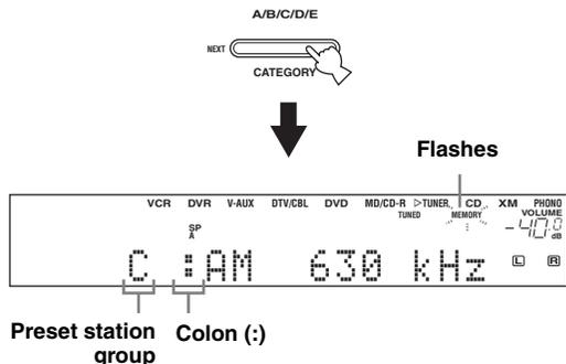
**4 Press PRESET/TUNING/CH </> to select a preset station number (1 to 8) while the MEMORY indicator is flashing.**
