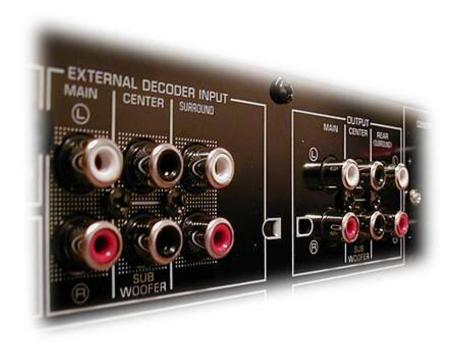
Levels should be straightforward for most: Center, Left Surround, Right Surround, and Subwoofer are adjusted to match the Mains in level. Use your trusty Radio Shack SPL meter and the built-in test tones (or suitable external set such as may be found on Video Essentials) and match the 5 (or 6) channels.
