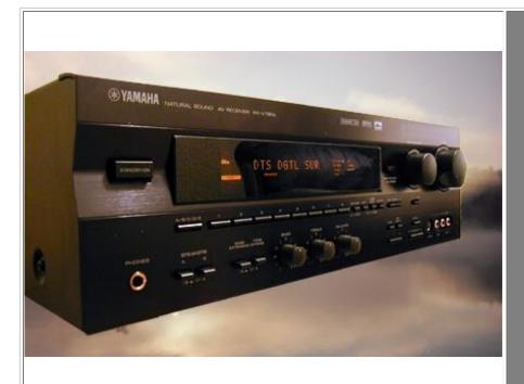
5.1 channel A/V receiver featuring Dolby Pro Logic, Dolby Digital, and DTS surround decoding in addition to DSP processing
