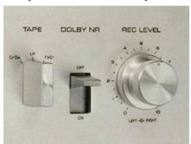
The Dolby system cuts tape hiss-noise for clear, beautiful music performance in the quietest passages. Even without using the Dolby circuit, the TC-511S boasts a full 53 dB signal-to-noise ratio. But with the Dolby switch on, there is a further 8 dB increase at frequencies above 5 kHz.
