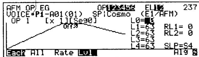
Move the DATA ENTRY slider up and down to modify any parameter that happens to be selected. The voice data has now been edited, and this is indicated by the small square being replaced by an inverse "E".
